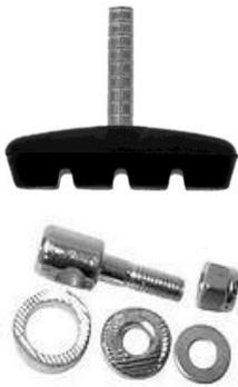
Most cantilever brakes have pads and hardware as pictured on the left, but some use V-brake pads. The traditional pads are difficult to adjust as they require an allen wrench and a hex wrench to tighten. The design also allows for pad adjustment in all three dimensions.
