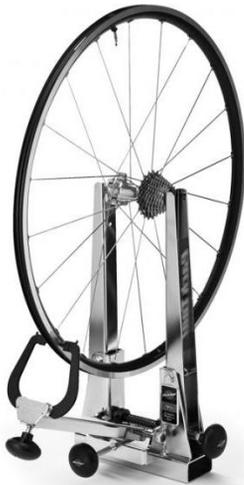
2) Spin the wheel and tighten the calipers until you locate the most severe (largest amplitude) bend in the rim. The calipers should ONLY hit the rim in one spot.
