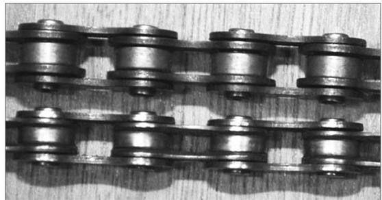
Singlespeed chain (top) versus multispeed chain (bottom)
