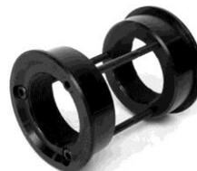
With this you can use any three-piece bottom bracket with standard threads
